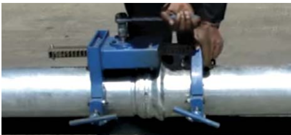
Easy to assemble and dis-assemble, Use pulling tools for big OD pipes.
